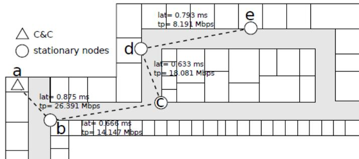
Figure 6: Approximate node positioning. Triangle is the fixed sink, circles nodes can be rearranged until satisfactory path characteristics are found.
