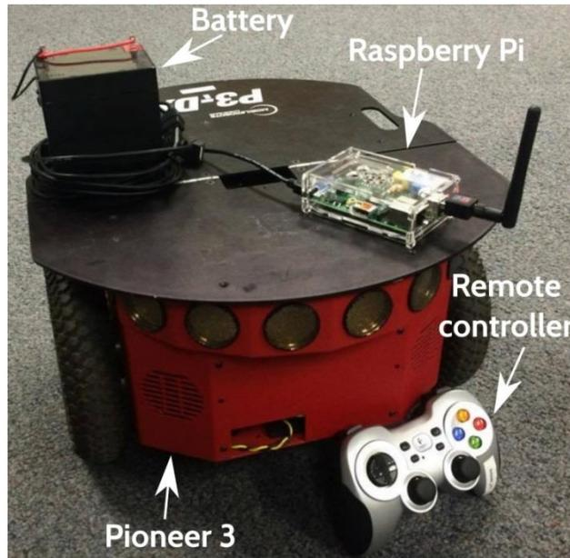
Figure 3: Mobile node hardware.
